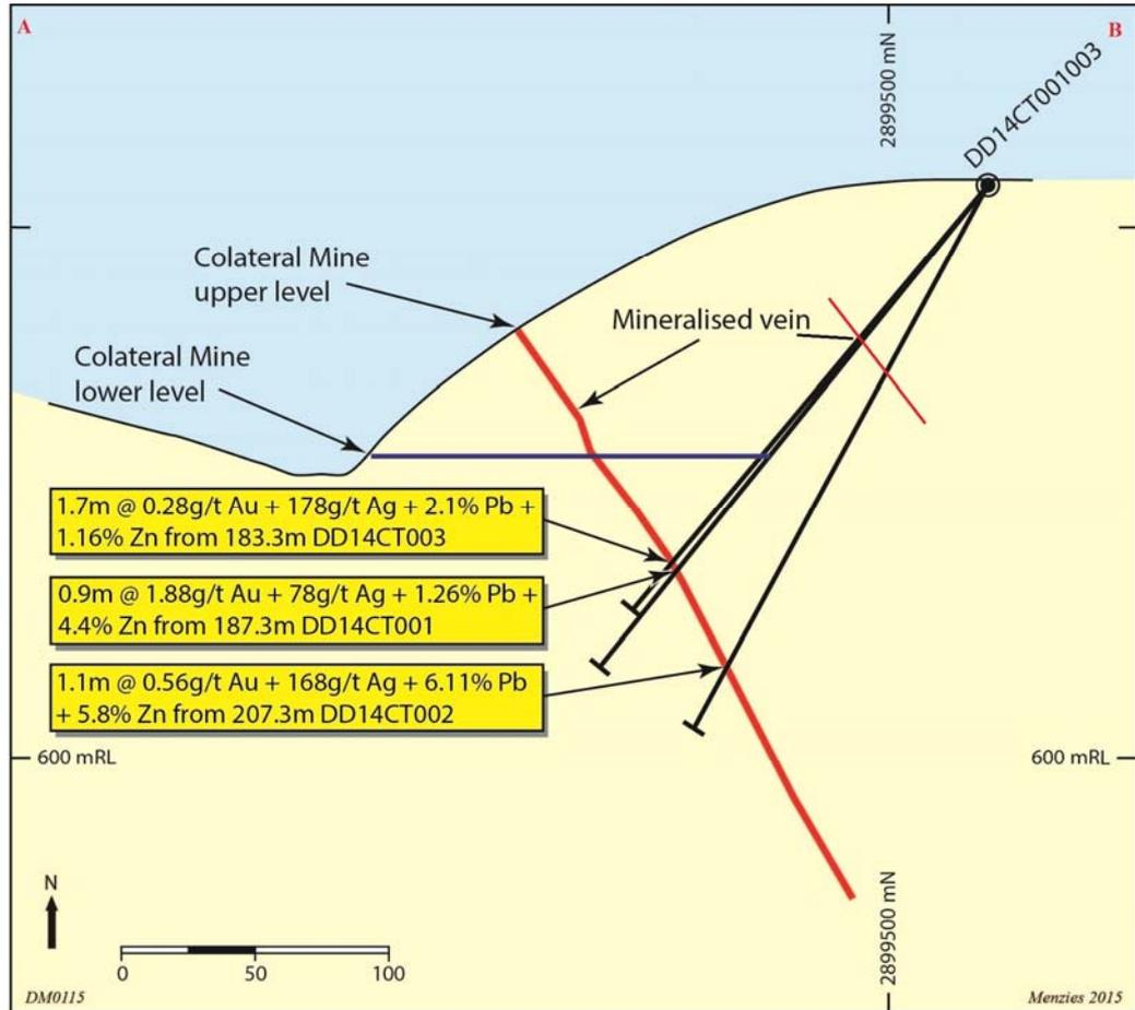
**Figure 1: Cross-Section: DD14CT001 – 003 intersecting the Colateral vein**
