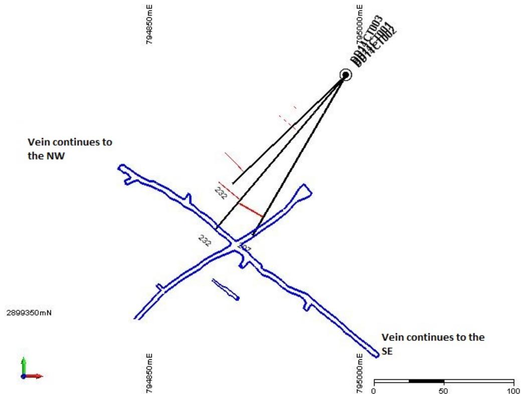
**Figure 2: Drill Hole Location & Plan Projection of Colateral Vein intercept points (red) below historic drift**
