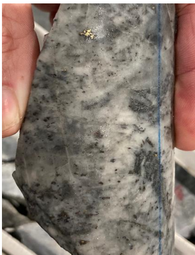
FIGURE 2: RAS CORE ILLUSTRATING VISIBLE COARSE GOLD
